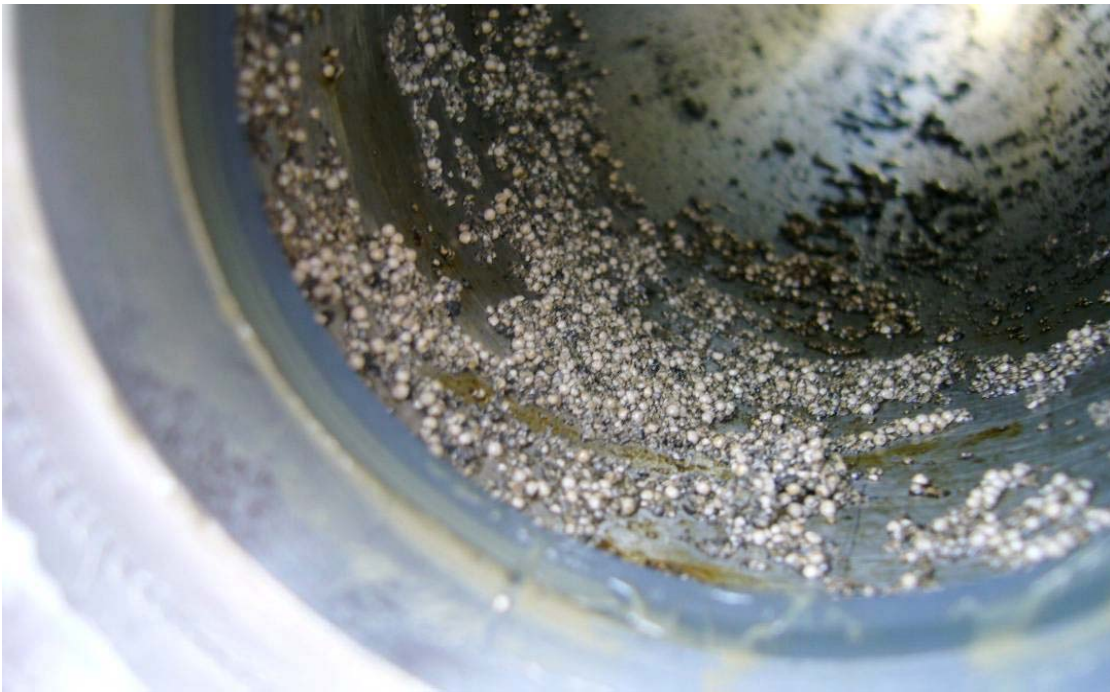
Figure 3 West Africa - Proppant can severely damage oilfield components
