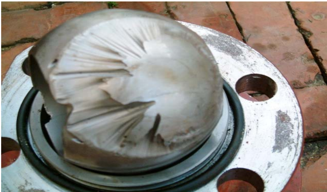
Figure 1 North Sea UKCS Example - Ball Valve exhibiting severe sand cut erosion
