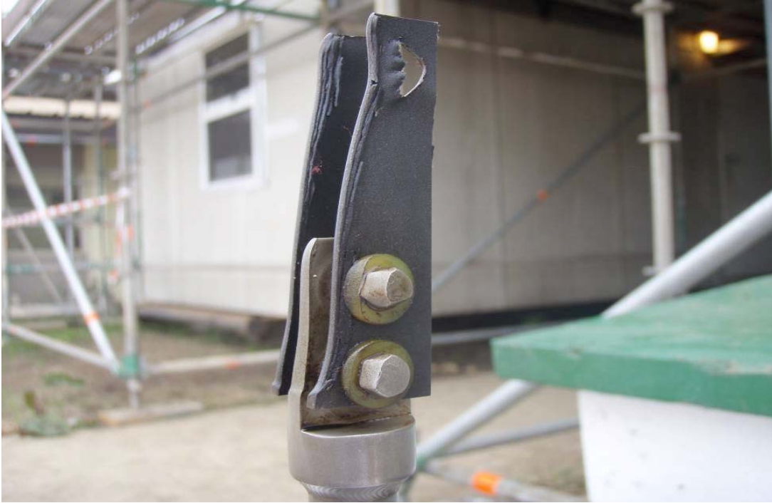
Figure 2 West Africa - Corrosion monitoring weight loss strip coupon displaying significant proppant induced erosion
